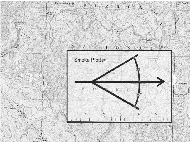
Figure D1 Smoke Plotter (NWCG RX 410)
